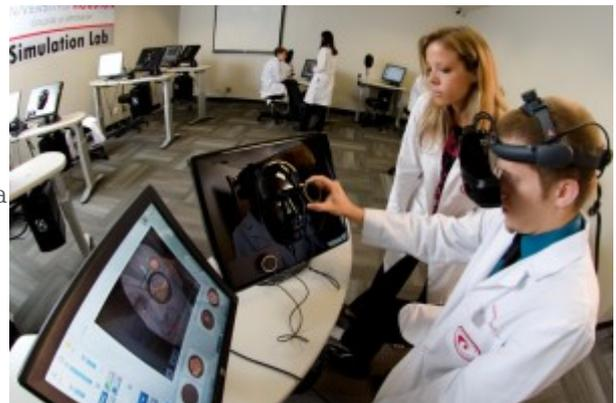
Image 1. A University of Houston College of Optometry student using the Eyesi Indirect simulator (VRmagic, Mannheim, Germany). Pictured are the touchscreen user interface, headband-mounted stereo display, handheld fundus lens and model patient face. Note that the student examiner views the patient images through the stereo display, while the touchscreen user interface simultaneously displays views for the on-looking instructor. [Click to enlarge](#)
