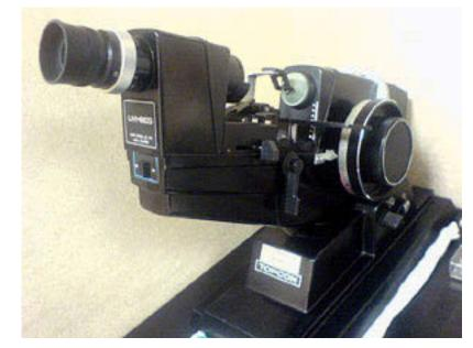
Figure 3 The analog knob on the manual keratometer seems to be a foreign entity to many Millennials.
